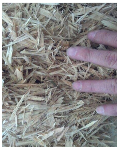
Figure 7 With the grain shavings (right photo) vs. across the grain shavings (left photo)
