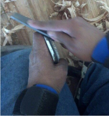
Figure 4 Sharpening the blade
