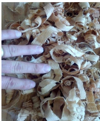
Figure 7 With the grain shavings (right photo) vs. across the grain shavings (left photo)
